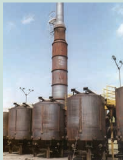
Metal kilns equipped with vapour incinerator for charcoal production in France
